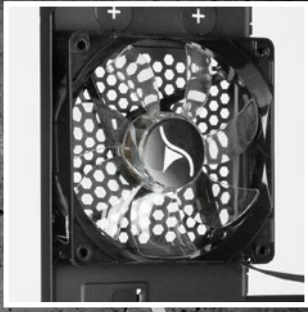
120 mm LED fan in rear panel
